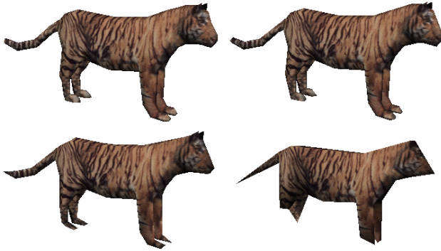
Fig. 2. Example for Progressive Meshes, the vertices numbers are 303, 203, 103, and 39 respectively
