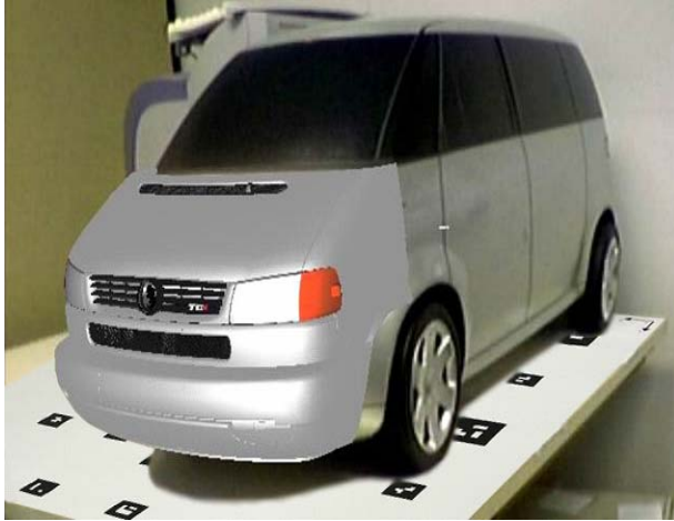
Fig. 1. Representation of a virtual front component of a VW Multivan on a real VW Microbus model
